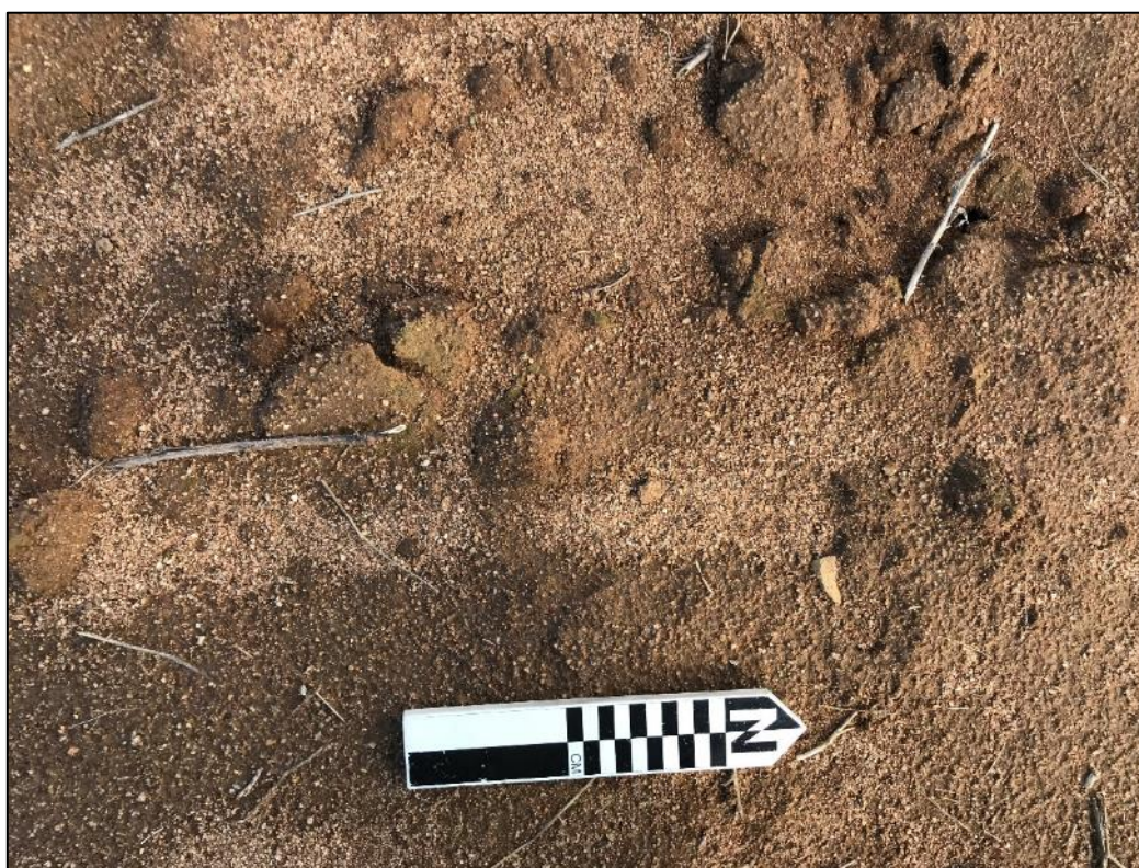
Figure 10. Representative photo of coarse-grained sandy loam in central portion of Project Area, plan view
